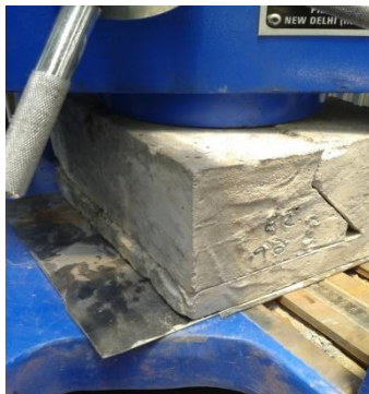
Figure 4: Interlocked Sample ‘b’ loaded parallel to bed-plane for Crushing strength
