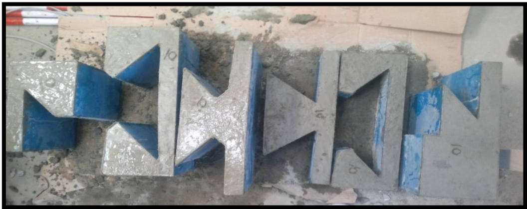
Figure 1. Interlocking Arrangement (male and female samples)
