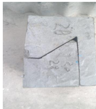
Figure 4: Interlocked Sample ‘b’ loaded parallel to bed-plane for Crushing strength
