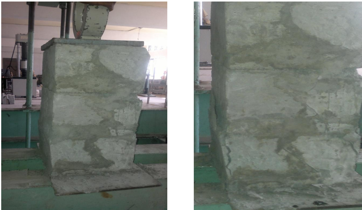
Figure 6: Prism wall with using mortar for interlocking before and after cracking (Sample "b")
