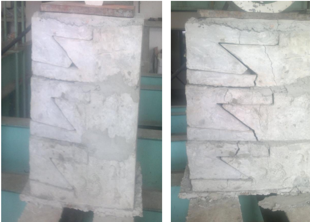
Figure 5: Prism wall without using mortar for interlocking before and after loading Sample 'a'
