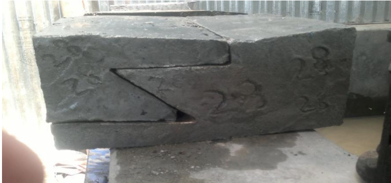
Figure 3: Interlocked Sample ‘a’ loaded parallel to bed-plane for Crushing strength
